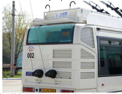
The driving equipment with three-phase inverter is designed to operate trolleybuses with two or three axles, supplied from the 750Vdc or 600Vdc overhead network. The power inverter is based on the IGBT transistors and is controlled by a DSP digital signal processor, which is using a vector flux control of the traction motor. By using adaptive control techniques a high level of comfort, rational usage of the traction motor and good control of the dynamics of the vehicle.
